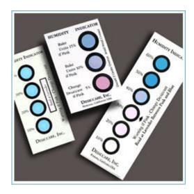
PPC carries a full line of Humidity Indicator Cards (HIC) which allows a low-cost method of indicating humidity conditions for various types of barrier packaging, including MIL Spec (MIL-I-8835) applications. The 30%, 40%, 50% HIC cards complies with MS 20003-2 and the 5%, 10%, 15% complies with JEDEC Standard 033. The 5%, 10%, 60% card complies with JEDEC Standard 033B.
